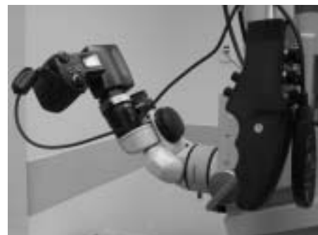
The afocal setup assembly is mounted on the microscope eyepiece, and the remote control is placed near the microscope control arm.
