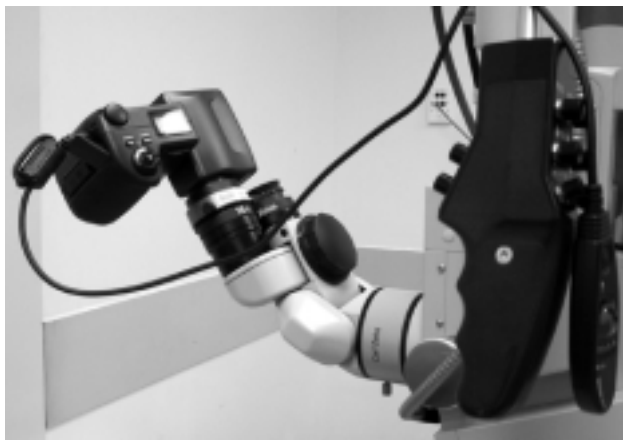
The afocal setup assembly is mounted on the microscope eyepiece, and the remote control is placed near the microscope control arm.
